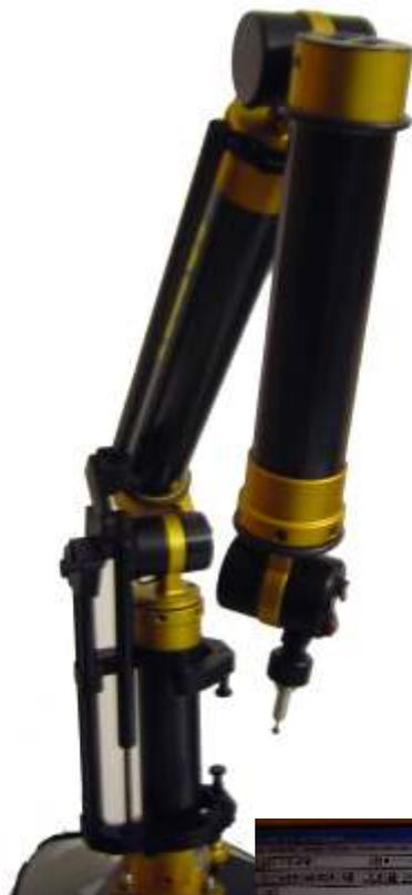
Using a **measuring arm** and two **measuring programs** (**nominal/actual value comparison** and **Best-Fit-methode**) before **delivery** we **check** the arrangement and **precision** of our gauges.
