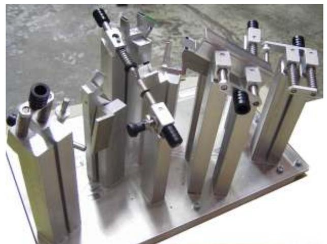
Gauge for controlling a pipe bundle with position control of fastening clip and angle.
