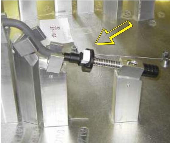
Control of the position and angle of the connector.
